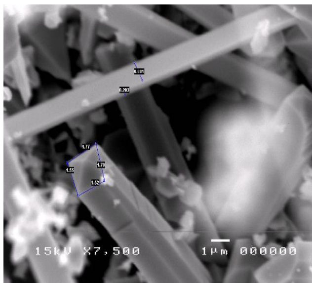
Fig. 1 SEM Image of the SnO 2 Nanomaterial grown at 1200°C for 1 hour
